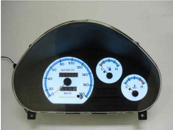
Fig. 9 Modified Dash Board including SOC Indicator
