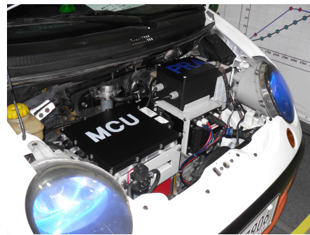
Fig. 12 Isometric View of EV Engine Room
