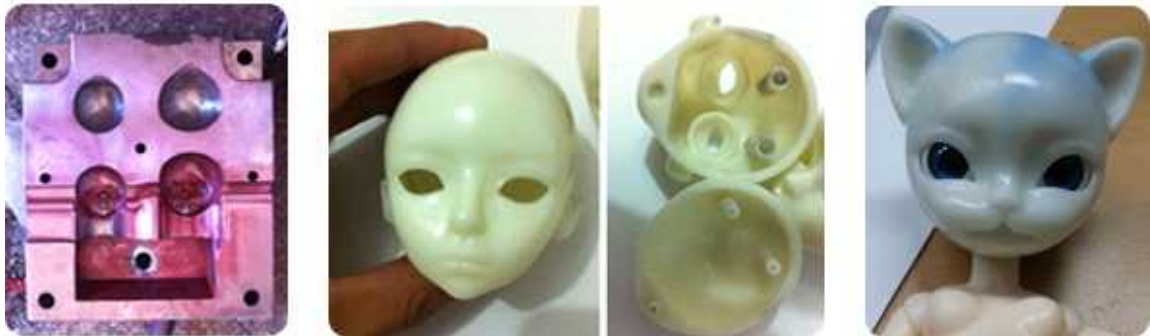
[Fig. 9] Example. The mold fabrication process to polygon data
