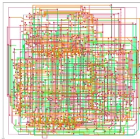
Fig. 3 Routed MCM-L BGA substrate
